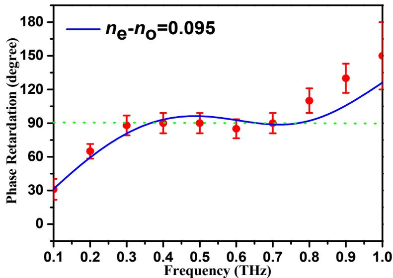
Fig. 5. The phase retardation of this device is about  $90^\circ$  from 0.30 to 0.70 THz, when  $\theta = 30^\circ$ .
