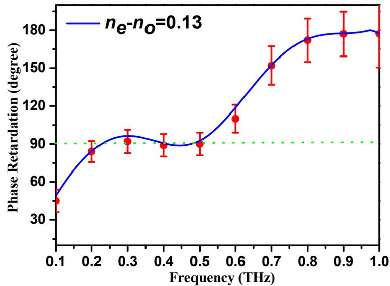
Fig. 4. The phase retardation of this device is about  $90^\circ$  from 0.20 to 0.50 THz, when  $\theta = 0^\circ$ .
