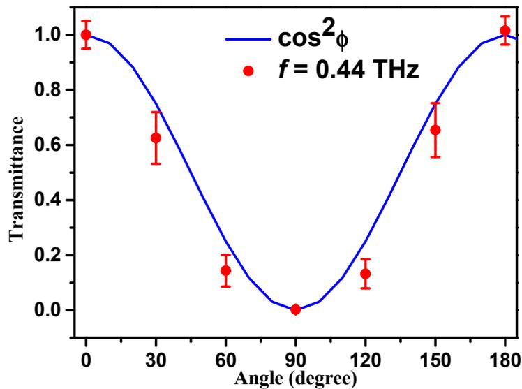
Fig. 3. The transmittance values with different  $\phi$  (when  $\theta = 0^\circ$ ) are drawn together with theoretic prediction at frequency of 0.44 THz.
