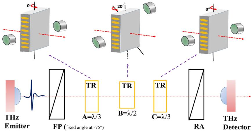
Fig. 1. The LC-based achromatic wave plate has three elements, A, B and C. Each tunable retarder (TR) consists of a pair of rotatable permanent magnets and a homeotropically aligned LC cell. The FP and RA represent polarizer with fixed angle at  $-75^\circ$  and rotating analyzer, respectively. Thicknesses of LC layers in  $TR_A$ ,  $TR_B$  and  $TR_C$  were  $d_A = 2.56$  mm,  $d_B = 3.86$  mm, and  $d_C = 2.56$  mm, respectively.
