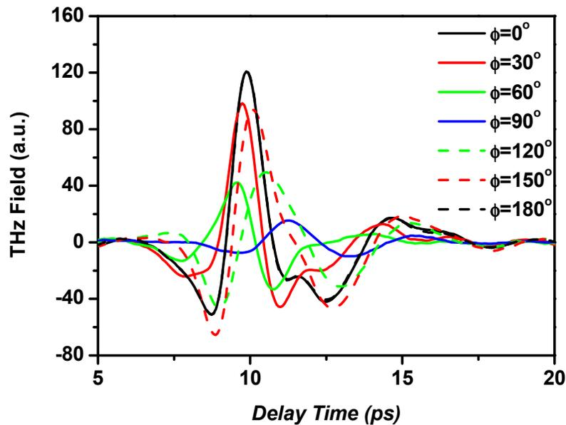
Fig. 2. The temporal waveforms of the THz pulse transmitted through the tunable achromatic quarter wave plate with the E7 layer aligned at magnetic inclination angle  $\theta = 0^\circ$  with different rotating angles  $\phi$  are shown together. Here we just show the temporal waveforms at  $\phi = 0^\circ$ ,  $30^\circ$ ,  $60^\circ$ ,  $90^\circ$ ,  $120^\circ$ ,  $150^\circ$ , and  $180^\circ$ .
